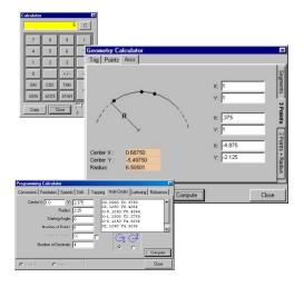
Calculate – Three calculators – programming, geometry and basic – are provided. The programming calculator provides major functions relating to feeds and speeds, drilling, tapping and lettering and displays user modifiable reference data. All calculators work with metric or English units.
