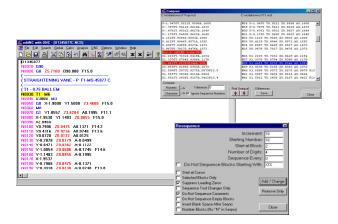
Edit – Functions to add, remove, or replace sequence numbers; reformat, scale, and transform coordinates; automatic selection of all blocks within a tool; basic lettering, smart Search; context-based help; user selectable fonts and colors.
